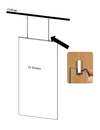
Screw Disc Code Screw Anchor to the ceiling along with wire rope. Repeat for the other suspension kit (\*do not install into plasterboard/ drywall unless with plywood reenforcement)
