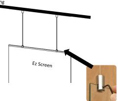
Screw Disc Code Screw Anchor to the ceiling along with wire rope. Repeat for the other suspension kit. (\*do not install into plasterboard/ drywall unless with plywood reenforcement)
